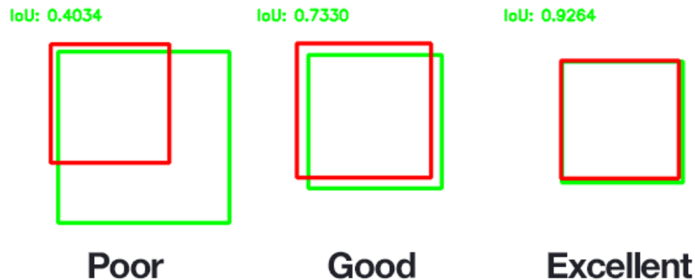
Figure 3: An example of computing Intersection over Unions for various bounding boxes.
